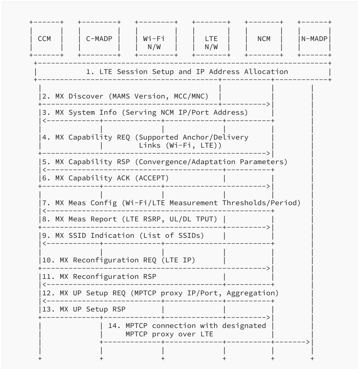
Figure 18: MAMS-Assisted MPTCP Proxy as User Plane - Initial Setup with LTE Leg
