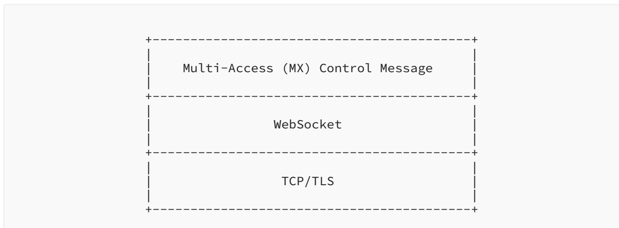
Figure 2: TCP-Based MAMS Control-Plane Protocol Stack
